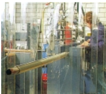
Strips provide for faster material flow and facilitate passage of the workpieces.
